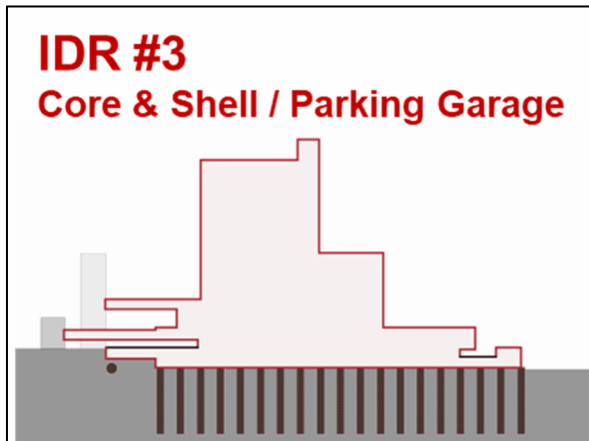
IDR 3: Construct the Exterior of the building as well as the core elements of elevators and stairs. Construct the parking garage.
