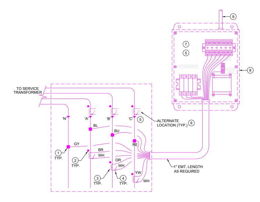
UTILITY METER-IN-A-BOX WIRING
