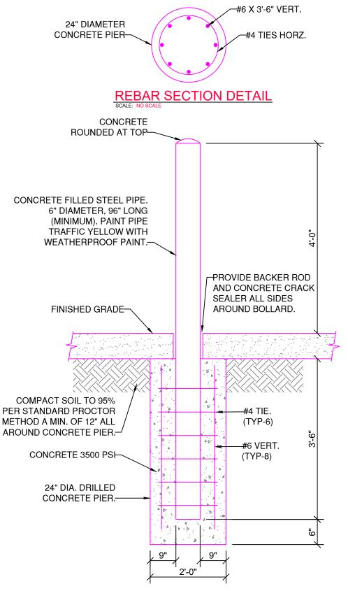
1 CONCRETE BOLLARD DETAIL
